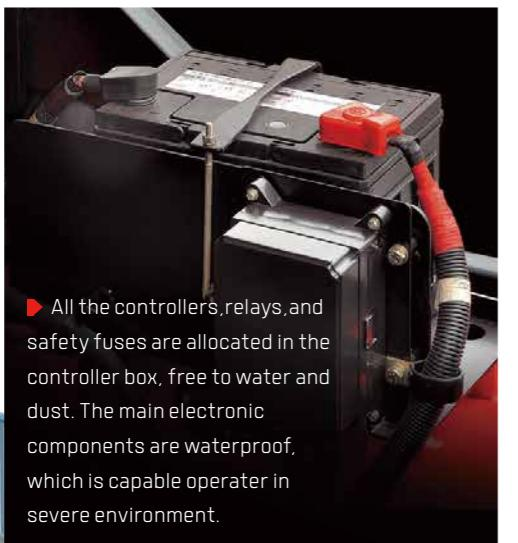
► All the controllers, relays, and safety fuses are allocated in the controller box, free to water and dust. The main electronic components are waterproof, which is capable of operation in severe environments.
