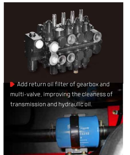
► Add return oil filter of gearbox and multi-valve, improving the cleanliness of transmission and hydraulic oil.
