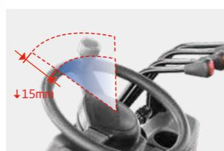
The small diameter steering wheel with tilt adjustment provides the ideal operating position. The superior responsiveness of the steering wheel optimizes maneuverability even in narrow spaces.
