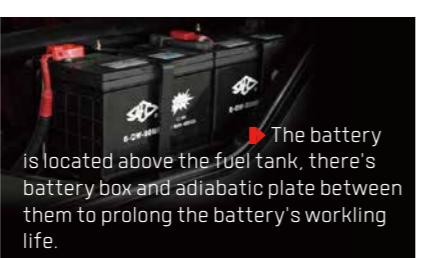
► The battery is located above the fuel tank, there's battery box and adiabatic plate between them to prolong the battery's working life.
