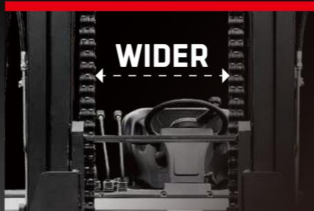
► The new design mast provides broad forward visibility due to outside located hydraulic pipes of fork positioner.
