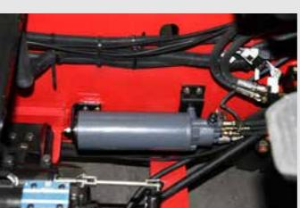
► There's an energy accumulator applied in the braking system, which means when the engine is shut down, it can also provide more than 4 times emergency brake.
