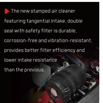
► The new stamped air cleaner featuring tangential intake, double seal with safety filter is durable, corrosion-free and vibration-resistant, provides better filter efficiency and lower intake resistance than the previous.
