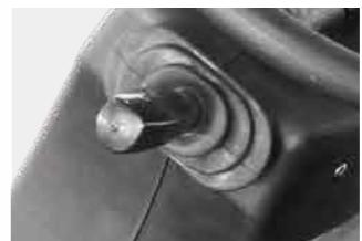
The new automobile-style light/turn-signal lever and forward-reverse lever are ergonomically designed and arranged to improve comfort and productivity.
